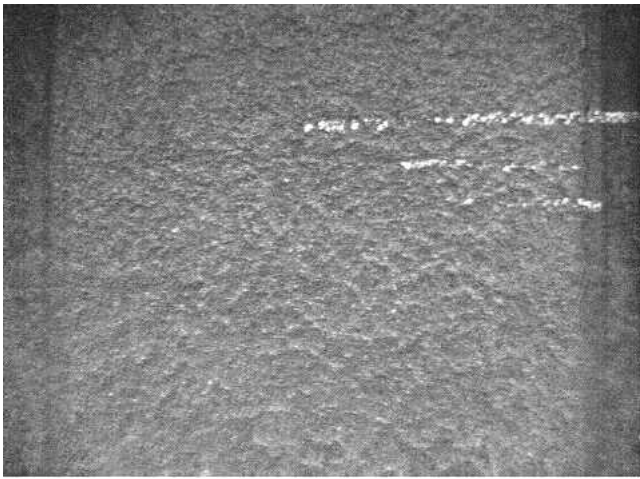
Fig. 7 Wear scar of the air plasma-sprayed conventional alumina-titania coating (the width of the wear scar is ~1.3 cm)
